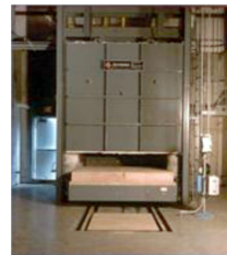
Car Bottom Furnace
